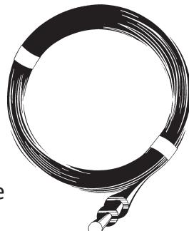
Lead-out is defined as the wire system that takes the power from the Energizer to the centre of the fence system - not just from the Energizer to the fence! Basically, the more wires connected in parallel, the better the voltage at the end of the fence.
